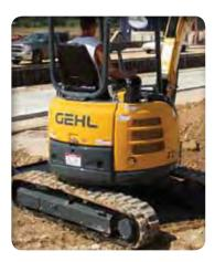
**TRUE ZERO-TAIL-SWING** design means no part of the upper structure overhangs the tracks during rotation. Cast side protectors provide added protection at the base of the house.
