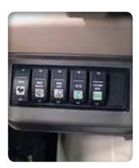
**ECO MODE** is activated with the flip of a switch, reducing engine speed by 10% without sacrificing power. This saves fuel when full speed is not necessary.
