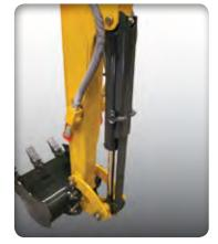
**EXTRA PROTECTION** on the bucket, dipper and boom cylinders is provided by plate spring cylinder guards. The upper structure's lower frame is reinforced by high-strength steel covers.
