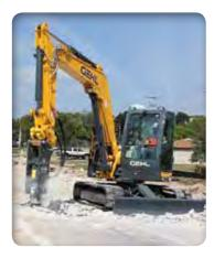
**ON-DEMAND HYDRAULICS** provide no loss of hydraulic performance during simultaneous movements, allowing smooth operation even while using the boom and arm during turning.
