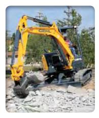
**ON-DEMAND HYDRAULICS** incorporate four hydraulic pumps which require less engine power and provide no loss of hydraulic performance during simultaneous movements.
