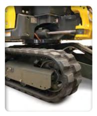
**EXTRA STABILITY** without adding to overall machine width is achieved with a wider track gauge and offset track drive system. Angled crawler frame reduces soil buildup.
