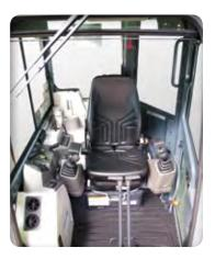
OVERSIZED CAB enclosure provides a spacious, ergonomic operating environment. The cab is mounted on five silicon oil filled isolators which reduce cab noise and vibration to the operator.
