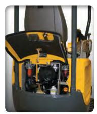
EASY SERVICEABILITY and simple daily maintenance checks are achieved through the removable side panels, large rear door and access panel under the operator seat.
