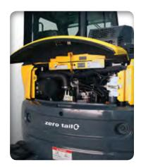
SERVICEABILITY and daily maintenance checks are made easy with the large removable side panels, flip-open rear engine door and under-seat access panel.
