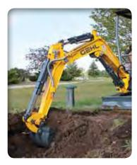
HIGH-PERFORMANCE BOOM is constructed with thick side plates and a single-pin mounted design for optimal strength and durability.
