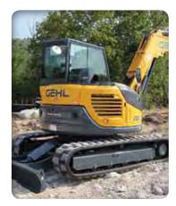
AUTO DECELERATION improves fuel economy and lowers noise and emissions levels by reducing engine speed to idle after four seconds without hydraulic movement.
